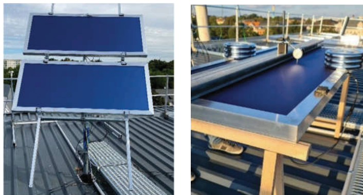
Fig. 5: Functional demonstrators installed in the solar laboratory (left) and frame load-deformation test (right)
