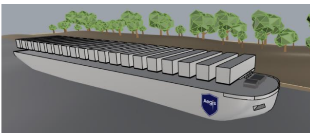
L_{oa}=85.0m | B=15.0m | T_{design}=2.5m Capacity: 38 Trailer
